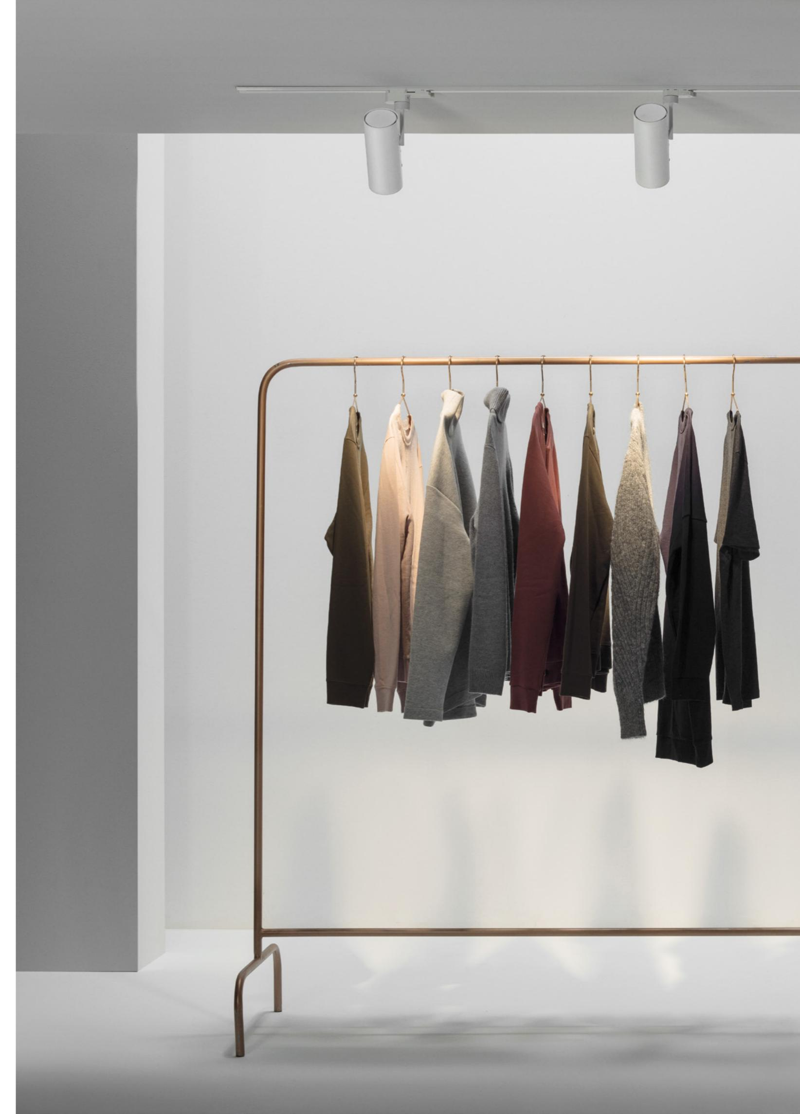
The flexibility of the three-phase rail installation allows the spotlights to be relocated according to the configuration of the space and the objects or areas to be highlighted.
